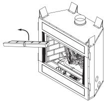
Figure 2 - Removing Front Refractory Access Panel
